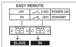
Easy Remote provides a simple way to remotely power-on/off the power amplifier. The Easy Remote function is only useful for appliances not employing a RCM-24 Module. Controlling appliances with RCM-24 Module installed per Easy Remote is practically pointless.
